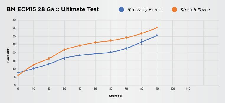
**Recovery Force:** Is indicative of the amount of compressive force a given film will exert on a unit load when applied at the listed strain conditions.
