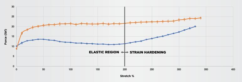
**Recovery Force:** Is indicative of the amount of compressive force a given film will exert on a unit load when applied at the listed strain conditions.
