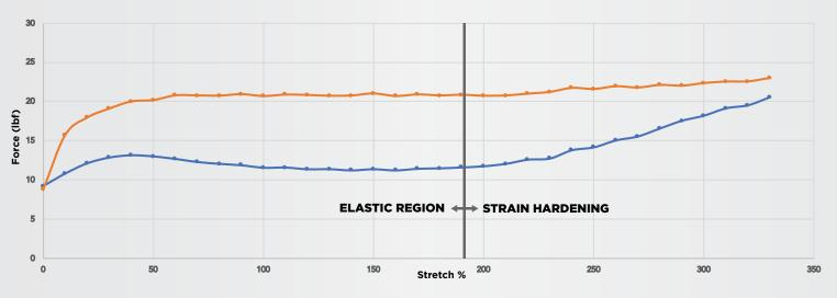
**Recovery Force:** Is indicative of the amount of compressive force a given film will exert on a unit load when applied at the listed strain conditions.
