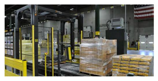
LoadLogic uses sensors to detect the dimensions and weights of variably sized pallets of products and automatically selects the appropriate stretch wrap pattern from nine preprogrammed, customized settings to ensure cost savings, material reduction, and containment consistency.
