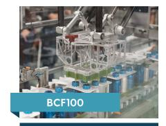
Fully automatic, high speed applicator; runs up to 600 cans/min
