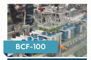
Fully automatic, high speed applicator; runs up to 600 cans/min
