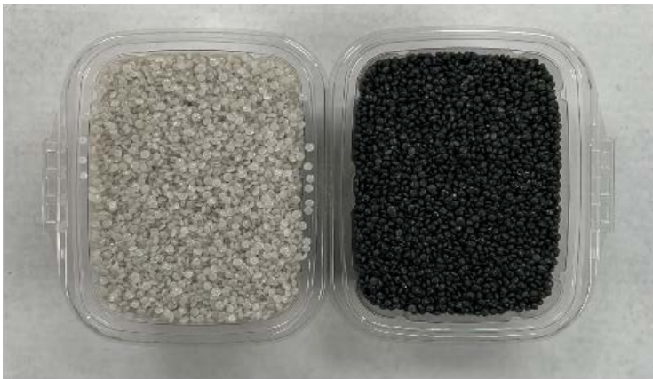
High-quality PCR resin (left) may be clear or have a grayish texture. Lower quality PCR (right) may be black due to contamination.
